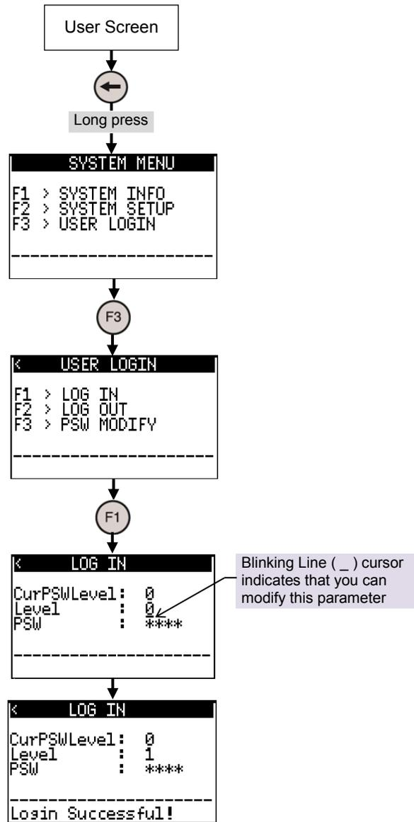
**i** Refer section [PSW Modify](#) to know the steps to enter password level and password value using HMI keys. User can modify individual digit. Selected digit is displayed and all other digits are masked by \* . Enter correct level and password and press Enter key to complete login.
