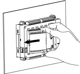
Push right side part of I/O extension unit towards Main unit till unit interface connector gets engaged with its male counterpart on Main unit. Projection provided on slot area on Main unit is accommodated through the oval shaped hole on PCB. Then push right side further gently till both the unit clips are clicked.
