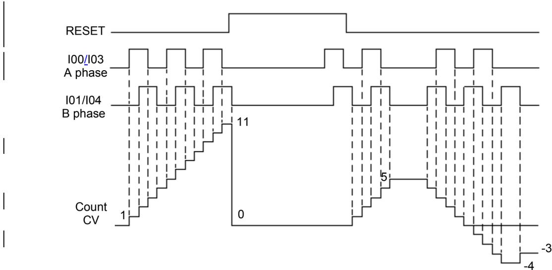
**Figure 36:** Functioning of AB encoder
