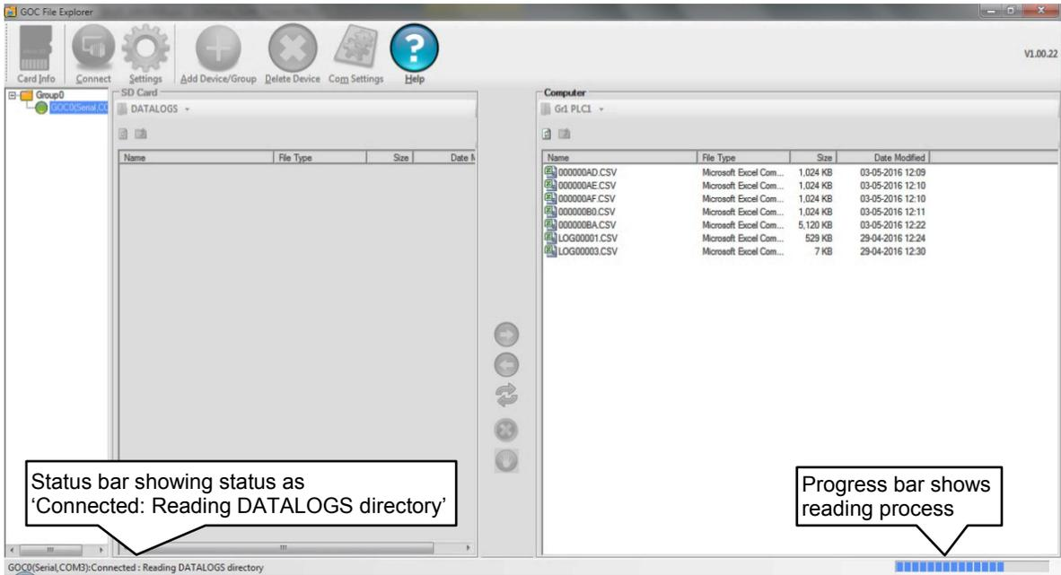
Status bar shows status as 'Device Name: Connected: Reading DATALOGS directory' and progress bar shows % of reading process.
