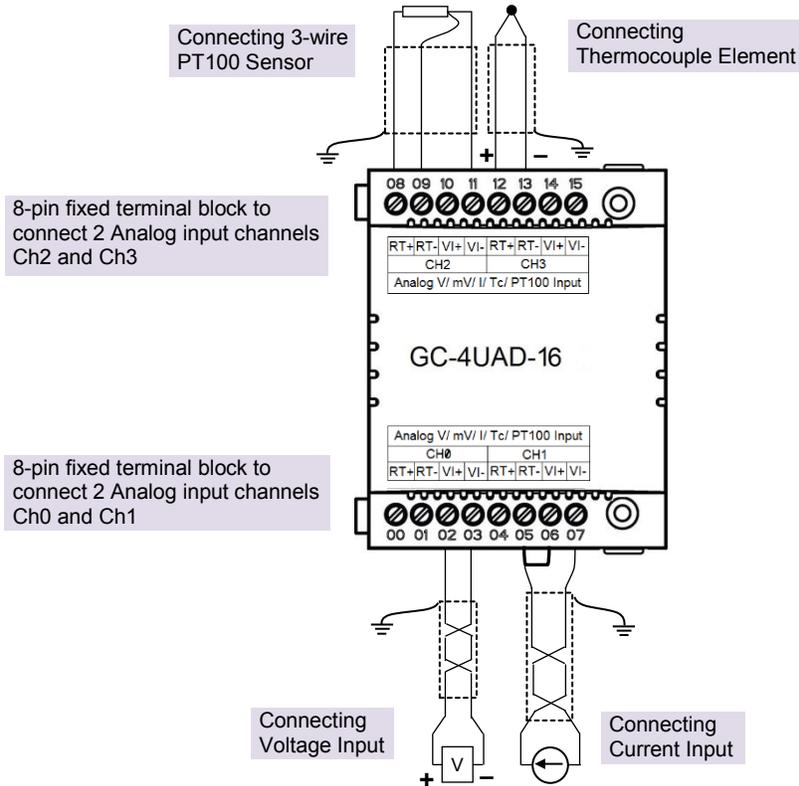
Figure 24: Wiring GC-4UAD-16
