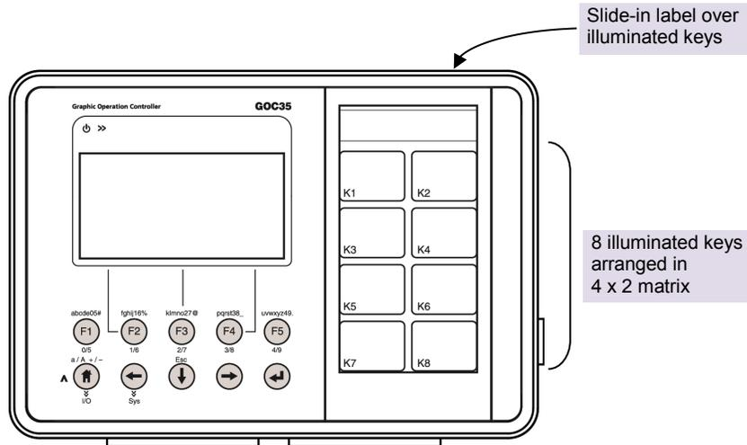
Figure 42: Illuminated keys with slide-in label
