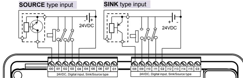
**Figure 13:** Main unit input connections
