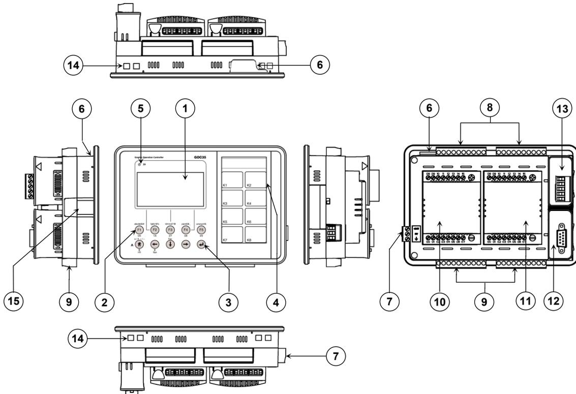
**Figure 4:** Main unit nomenclature with extension units
