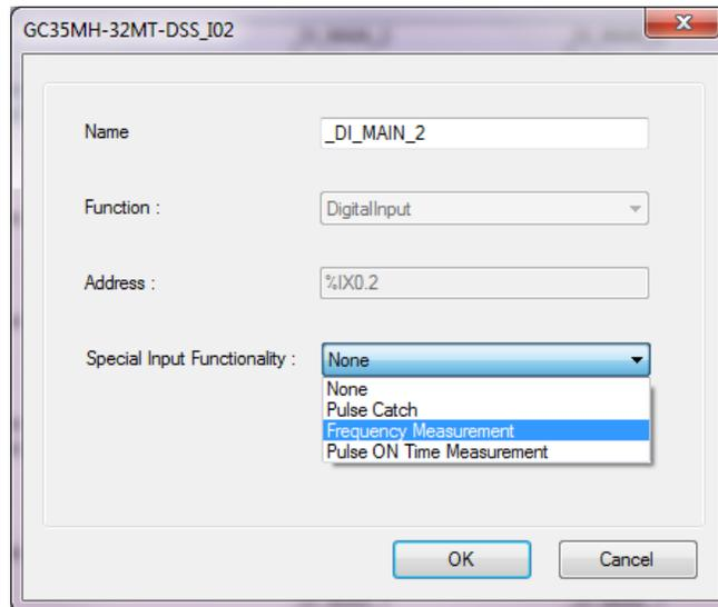
User can select “Frequency Measurement” and then set parameter “Minimum Frequency” in Hz from 0.1 to 50 Hz. Default value as 10.0 Hz.
