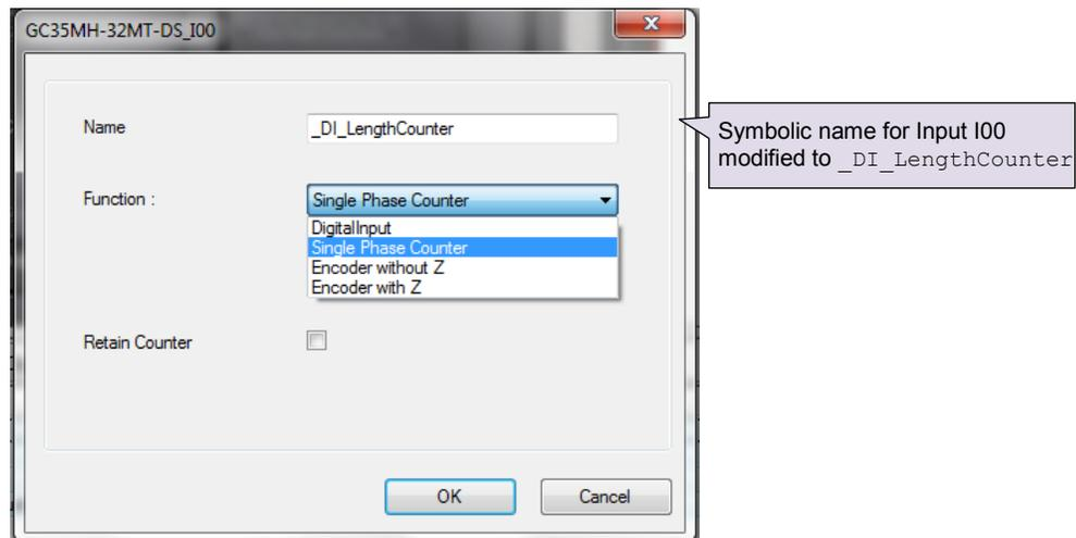
Based on this configuration, Hardware Configuration <R> generates a Global Variable List Implicit I/O List <R> which provides declaration of predefined global variables. The list below shows declaration of predefined variables for configuration of single phase counter.
