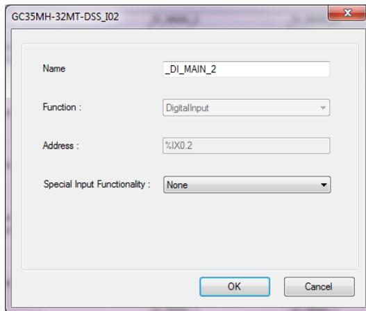
User can select special input functionality as “Pulse Catch” and can set parameter “Filter Time” in Hz with default value as 10000  $\mu$ s using drop-down list.
