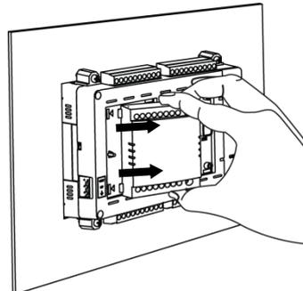
6. Ensure that cover is fitted on interface connector of unused IO slot.
