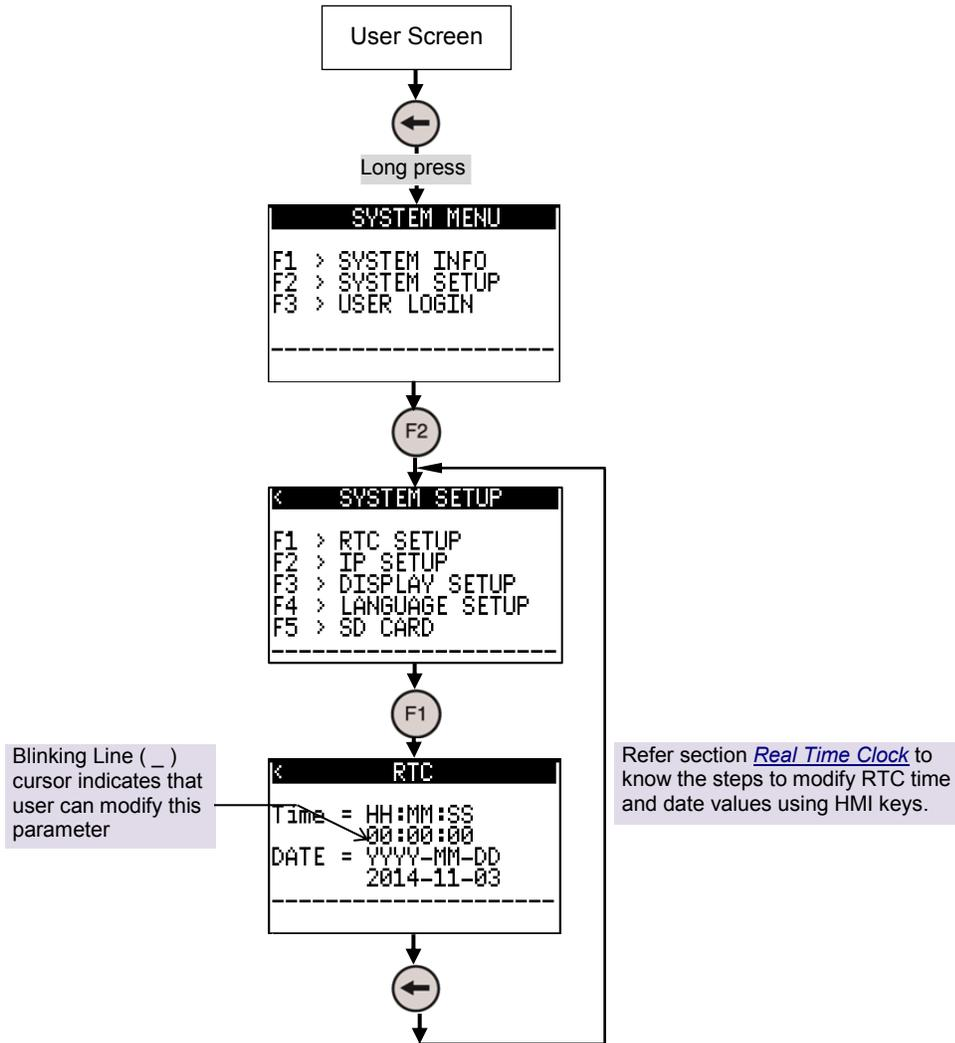
Refer section [Real Time Clock](#) to know the steps to modify RTC time and date values using HMI keys. When time and date entered is out of range, screen shows Error message momentarily as below.
