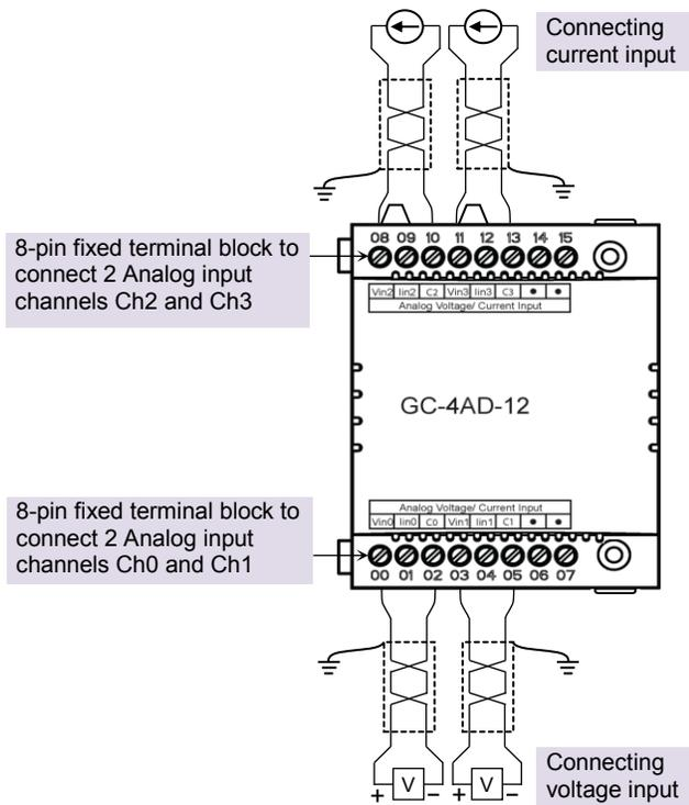
**Figure 20:** Wiring GC-4AD-12
