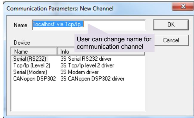
Select Tcp/Ip (Level 2) for Ethernet communication.
