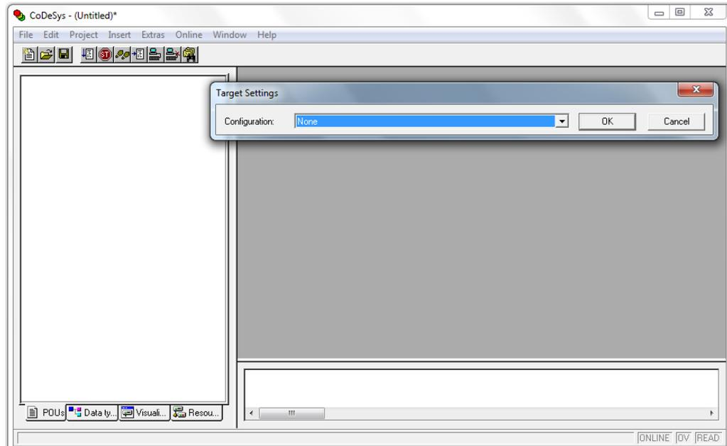
Select 'GOC target from Configuration drop down list and click on OK button as GOC35 Tm.n (Here, 'm' is 1 and 'n' is 0) as shown below.
