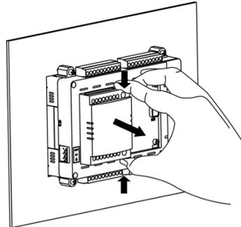
Slide I/O extension unit towards right side such that both latches on left side come out of respective openings on left side of slot area. Lift I/O extension unit away from Main unit to remove it from IO slot.
