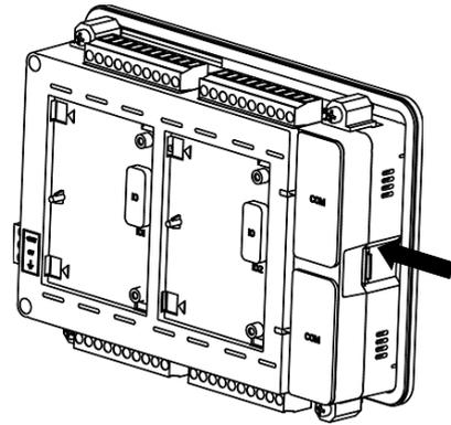
2. Locate SD card slot on side wall of Main unit.
