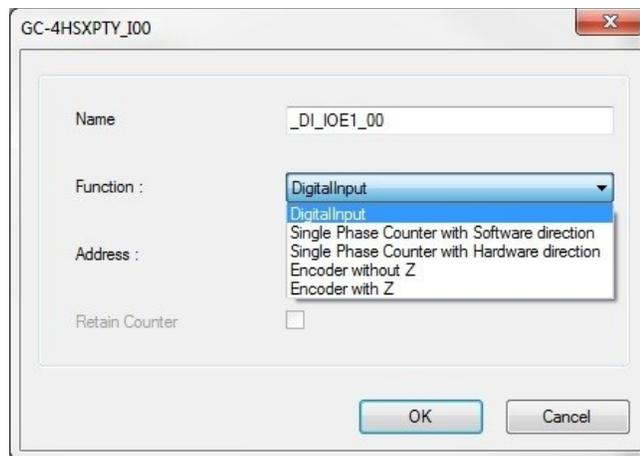
Based on this configuration, Hardware Configuration <R> generates a Global Variable List ImplicitIOList <R> which provides declaration of predefined global variables.
