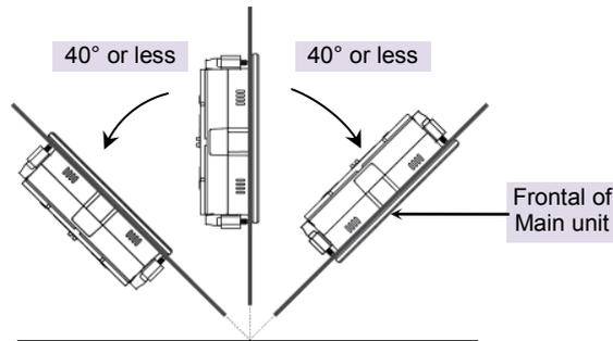
**Figure 9:** Mounting orientation
