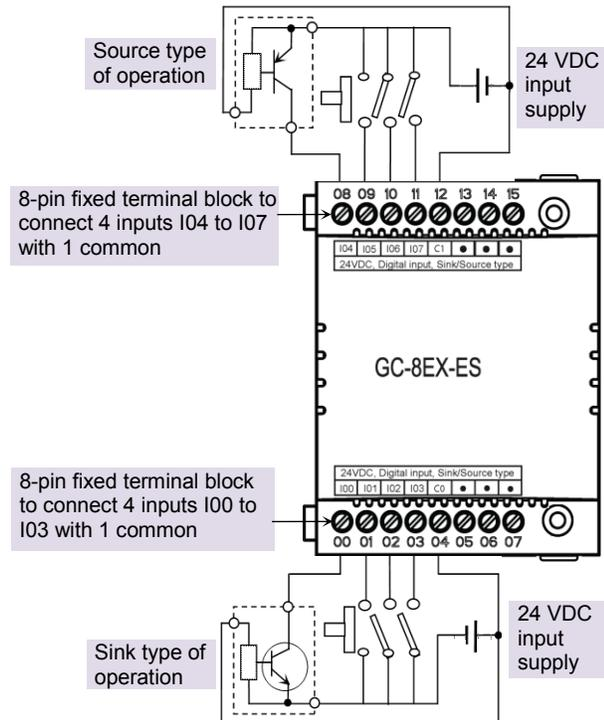
**Figure 17:** Wiring GC-8EX-ES
