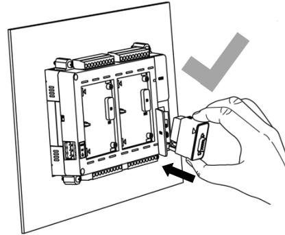
Firstly, insert bottom part of COM extension unit through slot
