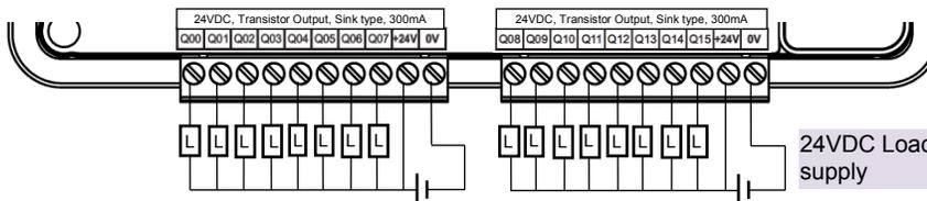
**Figure 14:** Main unit transistor sink output connections
