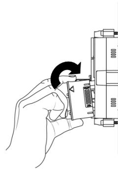
Then push upper part gently so that interface connector gets engaged with its male counterpart on Main unit.
