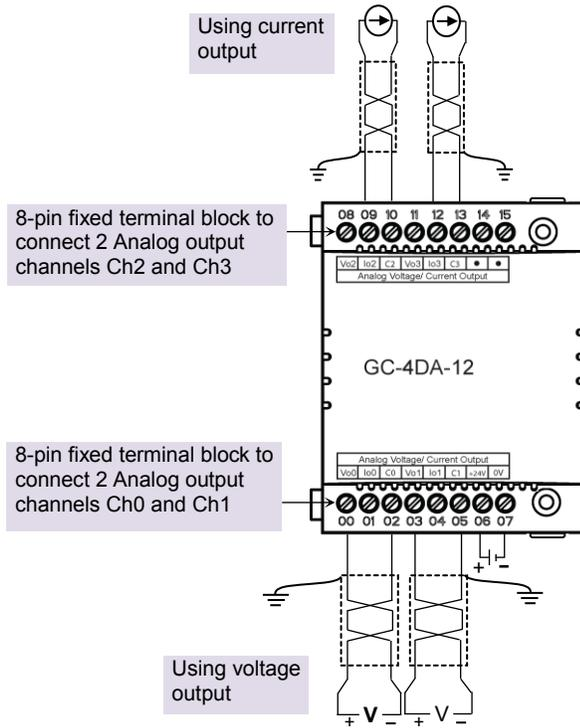
Figure 21: Wiring GC-4DA-12
