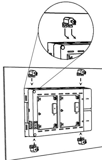
Turn mounting clamp screw in clockwise direction till tip of screw slightly touches inner surface of panel. Rotate screw an additional  $\frac{1}{4}$  -  $\frac{1}{2}$  turn in clockwise direction and ensure controller is firmly mounted in the panel. Fix all the 4 mounting clamps by tightening screws one by one progressively.
