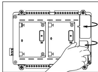
2. Prepare I/O extension unit for fixing
