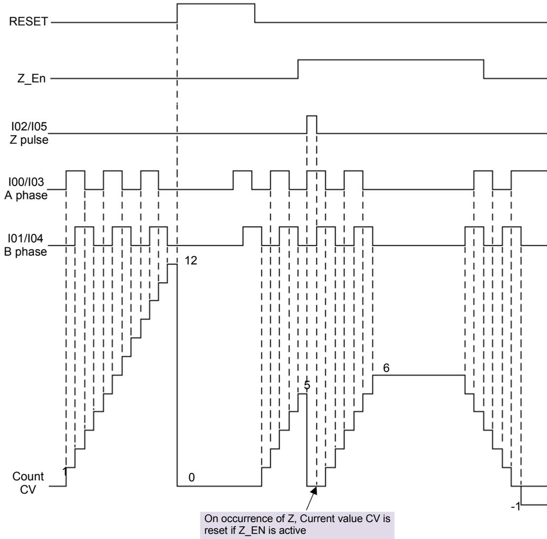
**Figure 37:** Functioning of ABZ encoder
