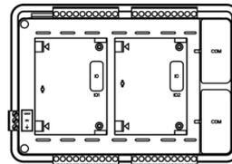
Remove interface connector cover on IO slot interface connector on Main unit.
