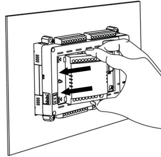
Insert both latches in respective openings on left side of desired IO slot (IO1/IO2) on Main unit and slide unit to left to insert latches completely inside openings.
