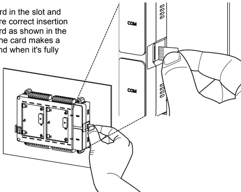
3. After correct insertion, SD card is detected and mounted automatically. Status can be monitored in system menu. Refer chapter '[System menu](#)'.
