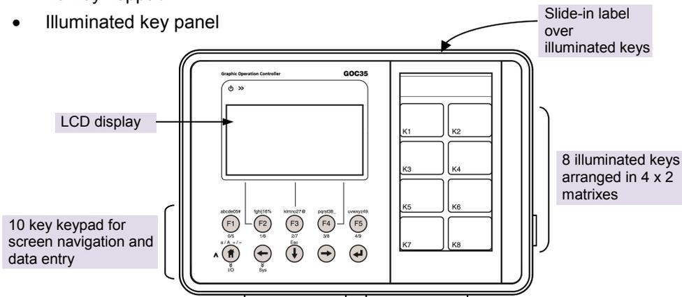
**Figure 39:** HMI components
