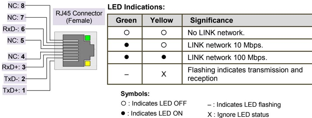
Figure 28: Connection details for GC-ENET-COM
