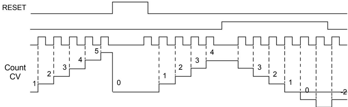
**Figure 34:** Functioning of single phase counter with software direction
