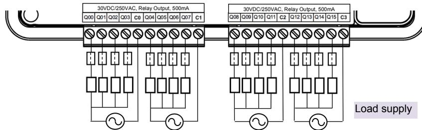
**Figure 166:** Main unit relay output connections
