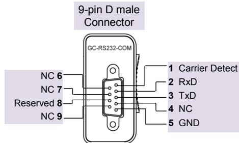
**Figure 26:** Connection details for GC-RS232-COM
