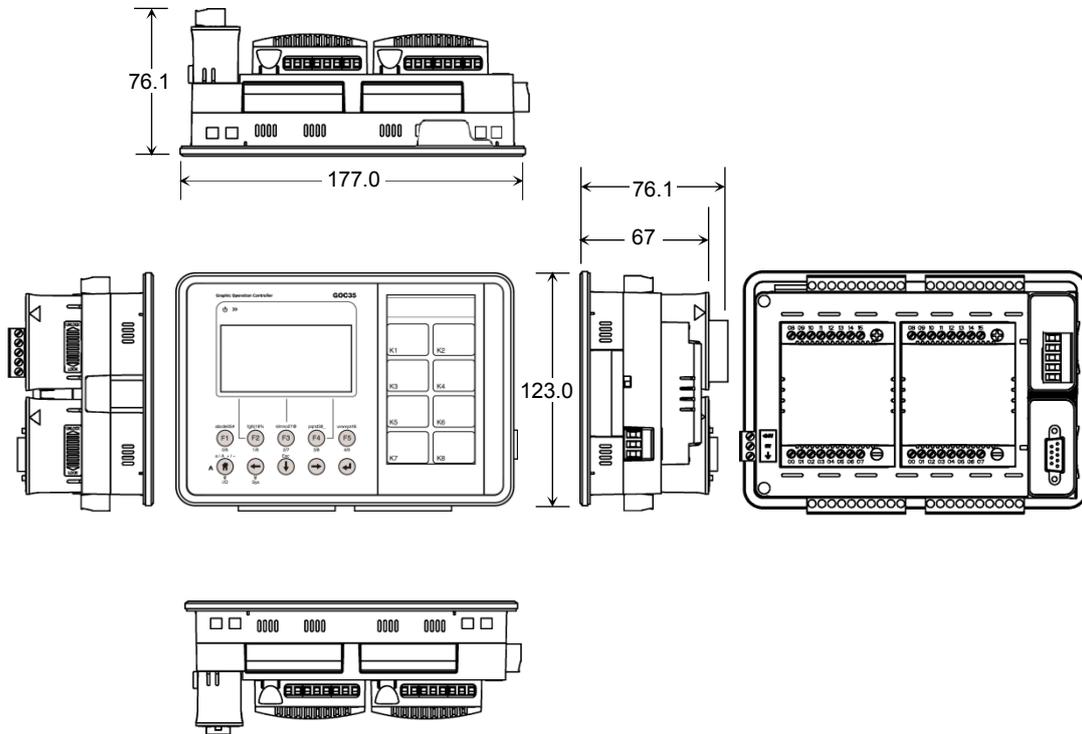
Figure 8: Main unit dimensions with extension units
