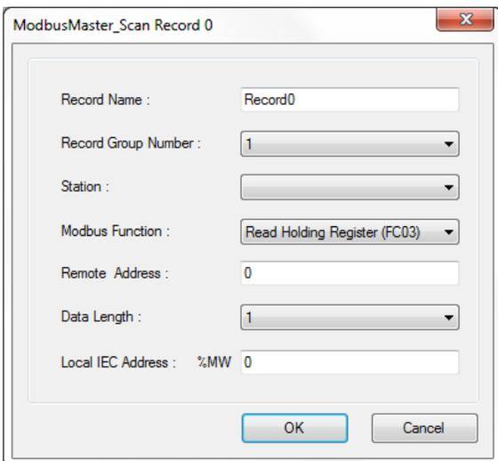
The table below provides the details of configuration required for Modbus scan record.
