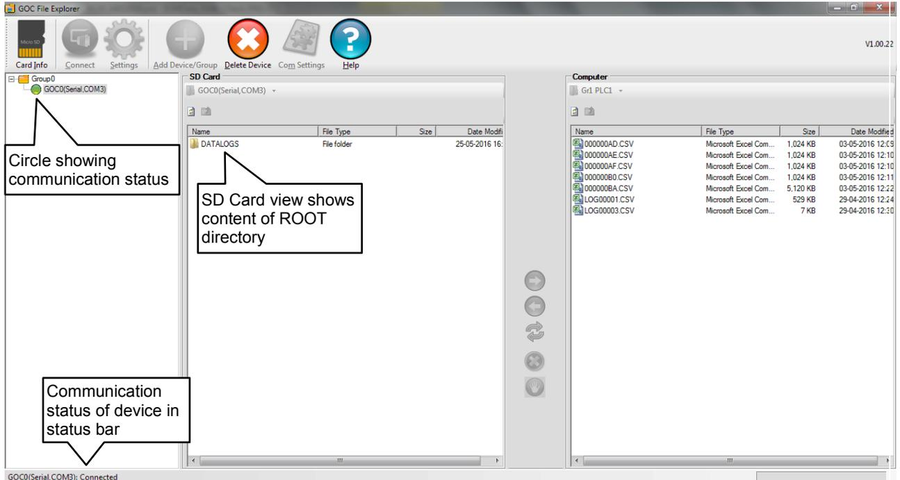
Note the circle in front of device in device explorer is now GREEN showing device is connected. Following table shows possible colors of the circle.
