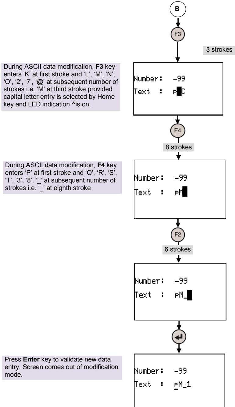
During ASCII data modification, **F3** key enters 'K' at first stroke and 'L', 'M', 'N', 'O', '2', '7', '@' at subsequent number of strokes i.e. 'M' at third stroke provided capital letter entry is selected by Home key and LED indication ^ is on.
