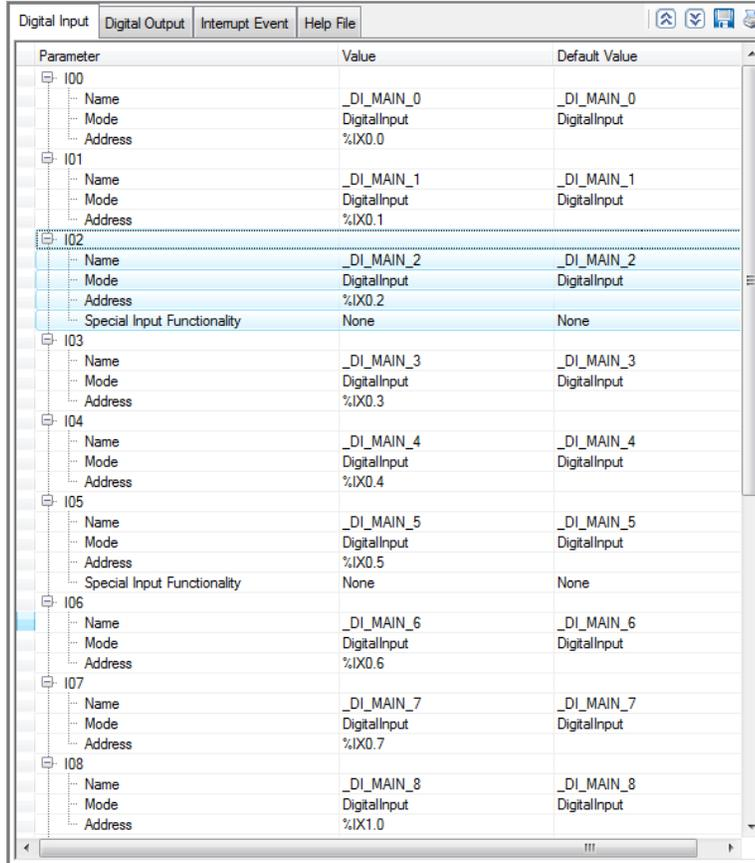
User can configure Pulse Catch functionality for digital input I02 and I05 by selecting respective input from "Digital Input" configuration tab and clicking on respective highlight.
