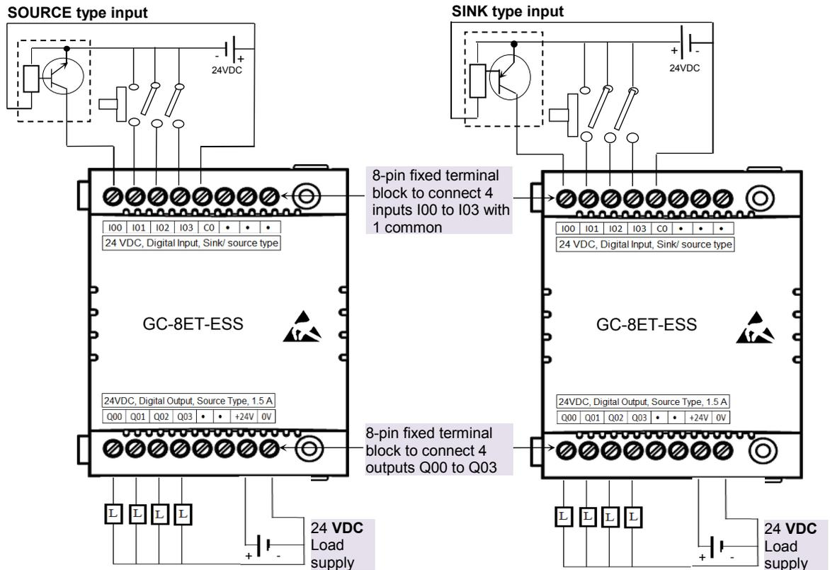
Figure 19: Wiring GC-8ET-ESS
