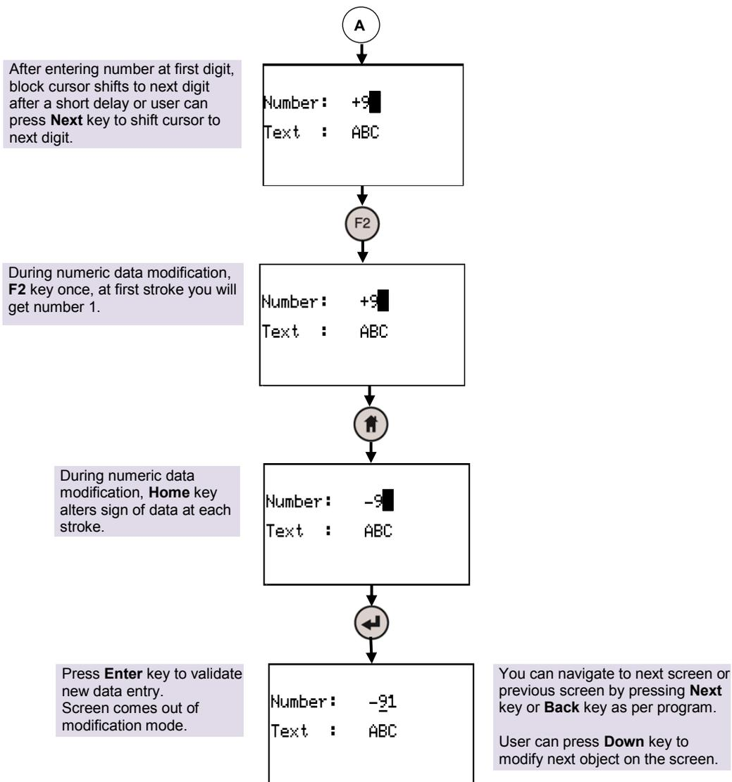
During data modification for any object (showing blinking block cursor at any digit), user can press **Down** key to come out of modification ignoring entry of new value. This will show line cursor blinking at first digit of the object under modification.
