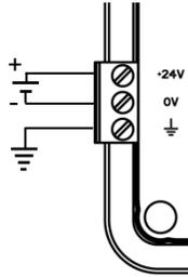
Figure 12: Main unit power supply wiring
