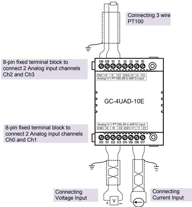
Figure 23: Wiring GC-4UAD-10E
