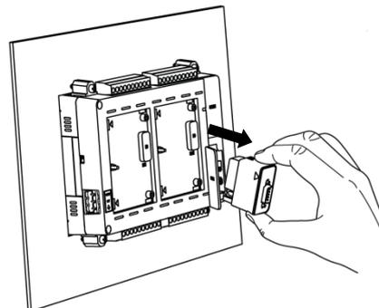
8. Ensure that cover is fitted on interface connector of unused COM slot.
