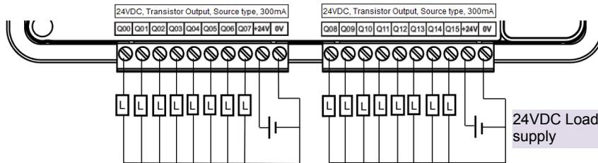
**Figure 15:** Main unit transistor output connections
