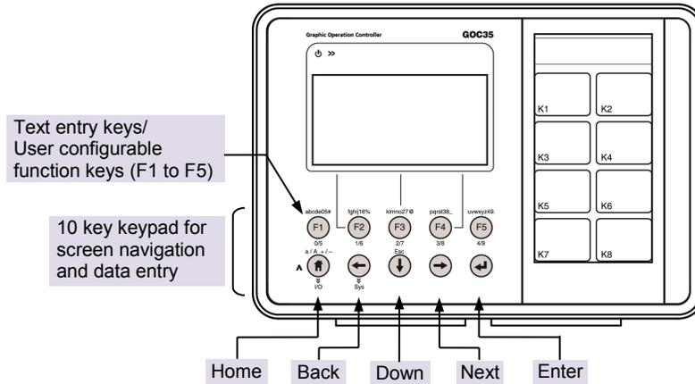
**Figure 40:** HMI keypad
