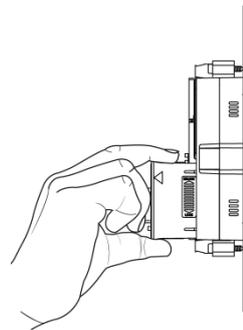
Push unit locking clip downward fully so that COM extension unit is locked firmly on the Main unit. Failing to do so will cause loose connection and sudden removal of COM extension unit from the slot.
