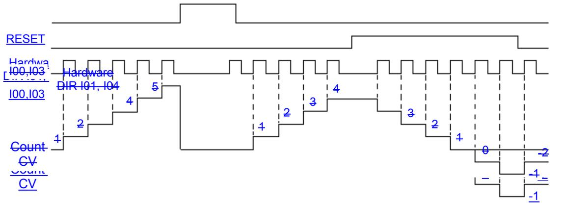
Figure 35: Functioning of single phase counter with hardware direction
