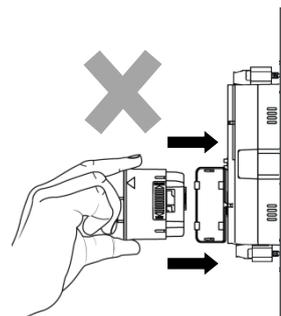
4. Insert COM extension unit in Main unit COM slot
