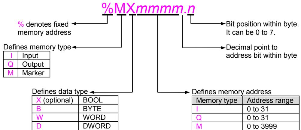
**Figure 31:** Addressing of PLC variables
