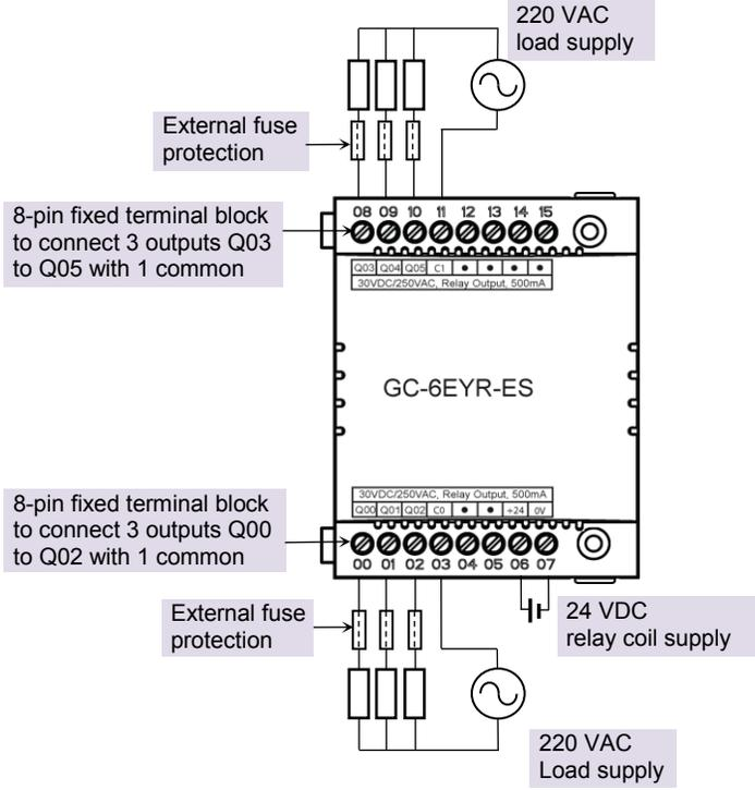
Figure 18: Wiring GC-6EYR-ES
