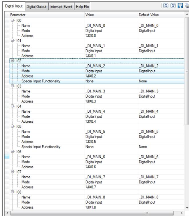
Select respective input from “Digital Input” configuration tab and click on respective highlight.
