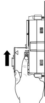
Keep thumb on bottom edge of front and pointing finger on top edge of front. Pull upper part of unit, so that its interface connector gets disengaged from its counterpart on Main unit.
